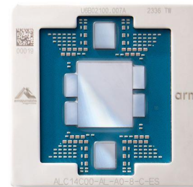
Amazon Data Center CPU 7 active chiplets
